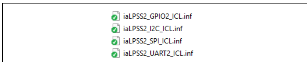
Figure 7. Serial IO Driver - INF files
